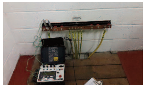
Bonding measurement performed onto Substation Earth Bar
